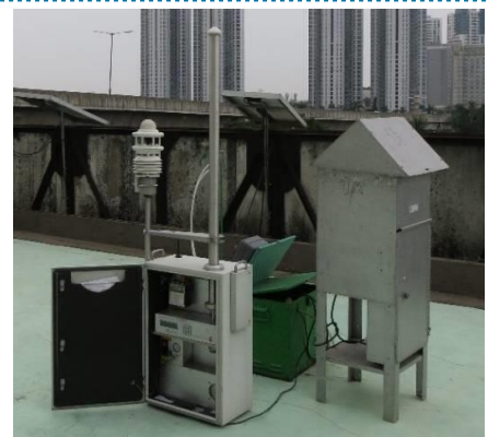
PM 2.5 monitoring equipment at BPLHD office
