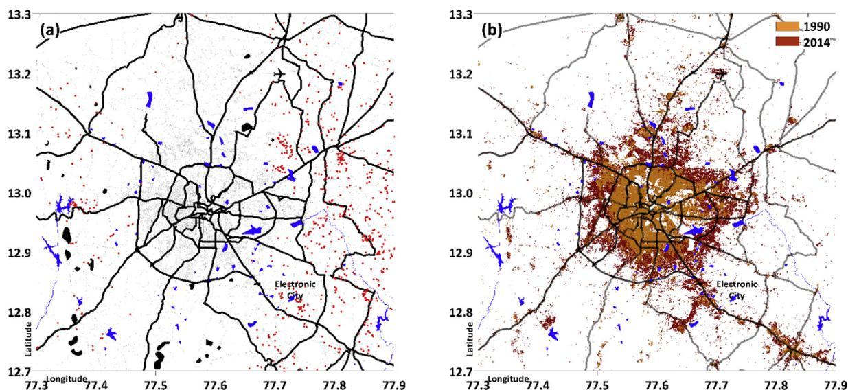
Fig. 1. (a) Selected urban airshed for the Greater Bengaluru region including main roads (thick lines), arterial roads (grey lines), water bodies (blue lines), airport (symbol), quarries (black patches), and brick kilns (red dots) (b) Urban built-up area in 1990 and 2014.
